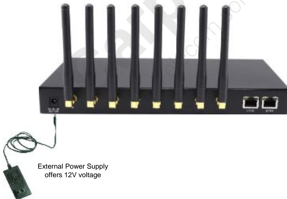
Figure 2-1 Wireless Gateway Power Connection
